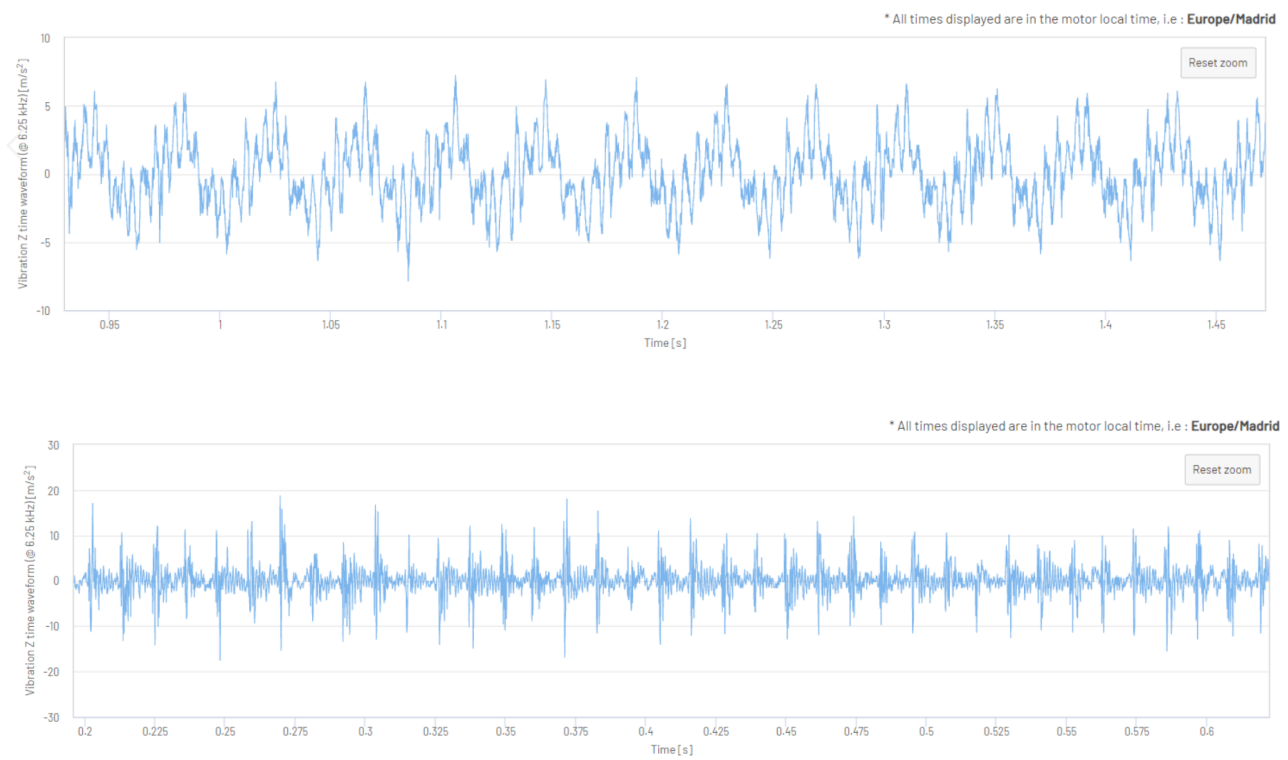
Figure 11 and 12: Vibration Z-Axis Time Waveform in \text{m/s}^2 (one 2.4 second sample, zoomed-in views)
