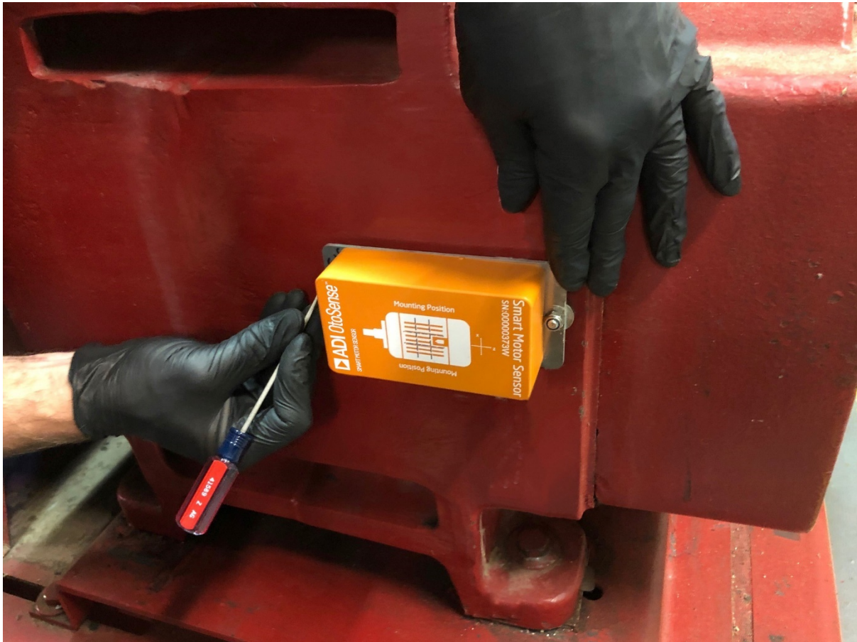
Figure 40. Installing an SMS device on a motor without cooling ribs
