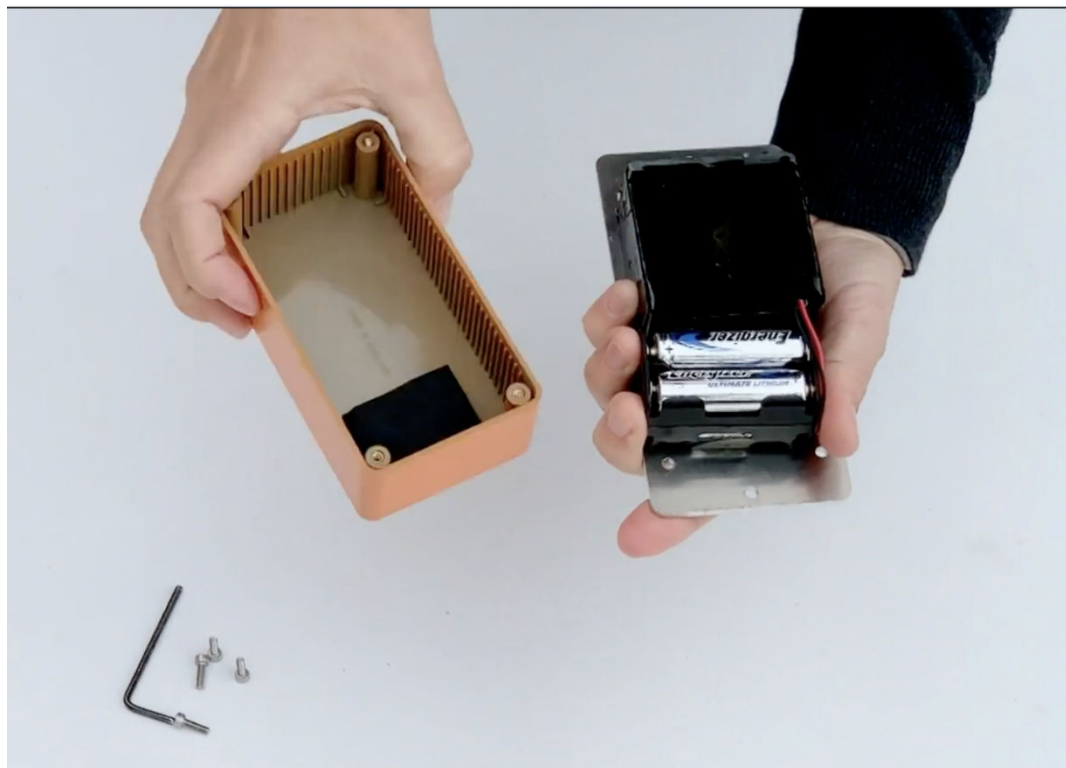
Figure 16. Position of the orange cover before re-inserting the screws
