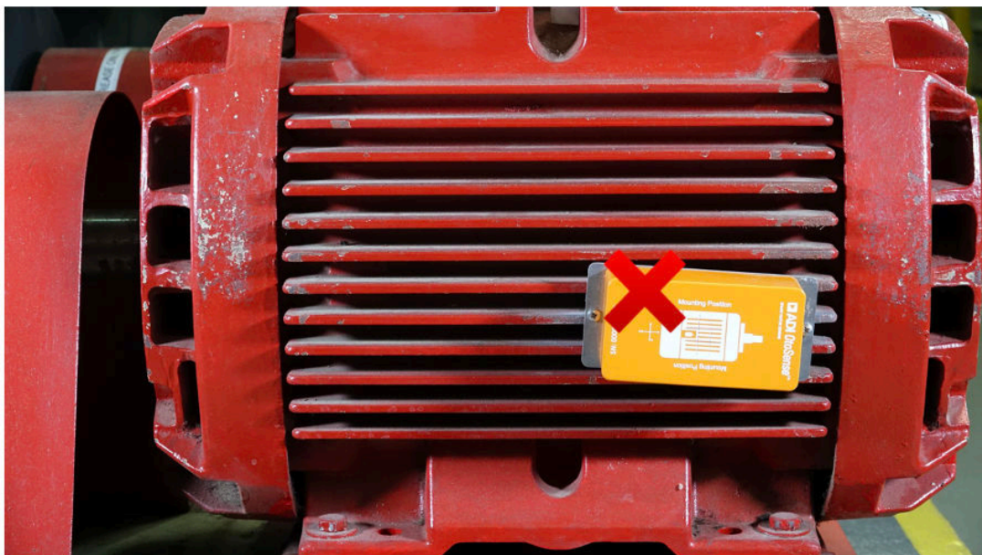
Figure 35. Incorrect Positioning – an SMS device laterally inverted with respect to the cooling shaft and not parallel to the cooling ribs
