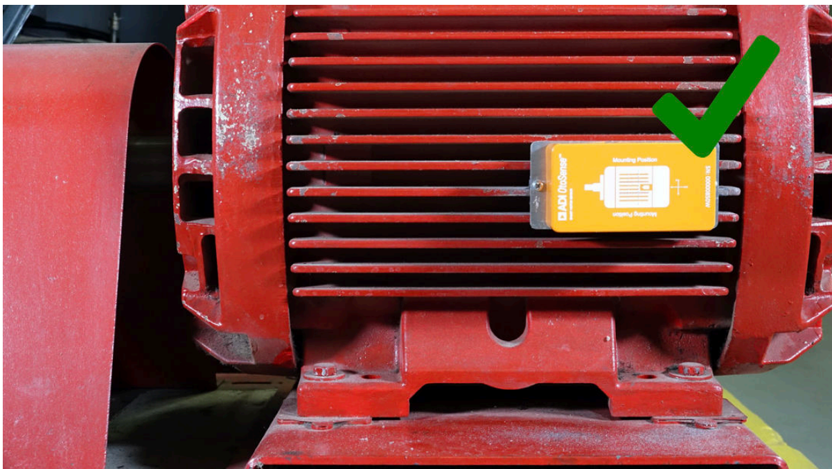
Figure 32. Correct positioning of the motor
