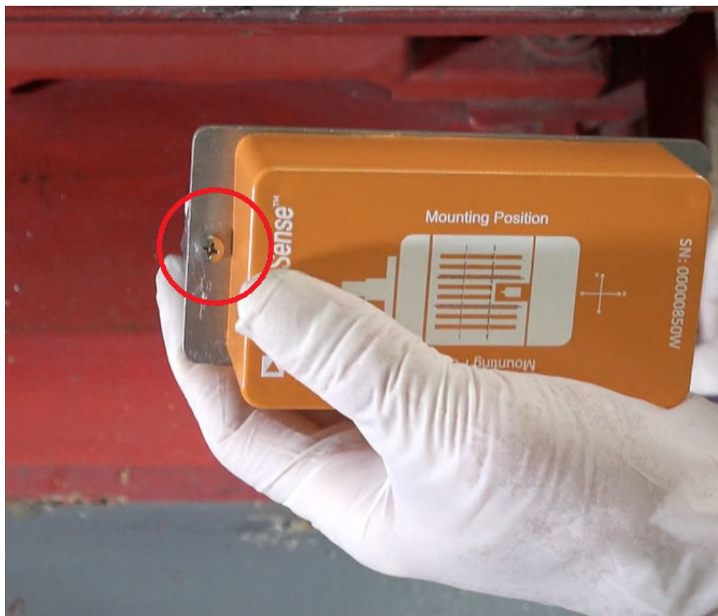
Figure 39. Position of the screws on the SMS device
